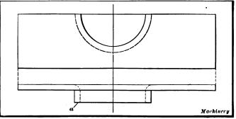
Fig. 38. A Drawn Cylindrical Projection
